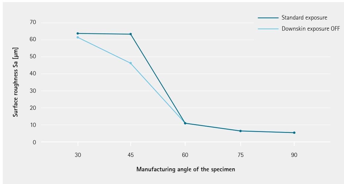
EOS NickelAlloy IN939 parameters were developed for optimized dimensional accuracy of internal cooling features, which are essential to hot gas path components in gas turbines. This comes with a compromise on downskin roughness. Whenever possible, for parts where optimized dimensional accuracy of internal cooling features is not needed, EOS recommends to switch off downskin exposure, to improve downskin roughness and buildability at low angles, and to increase process speed.
