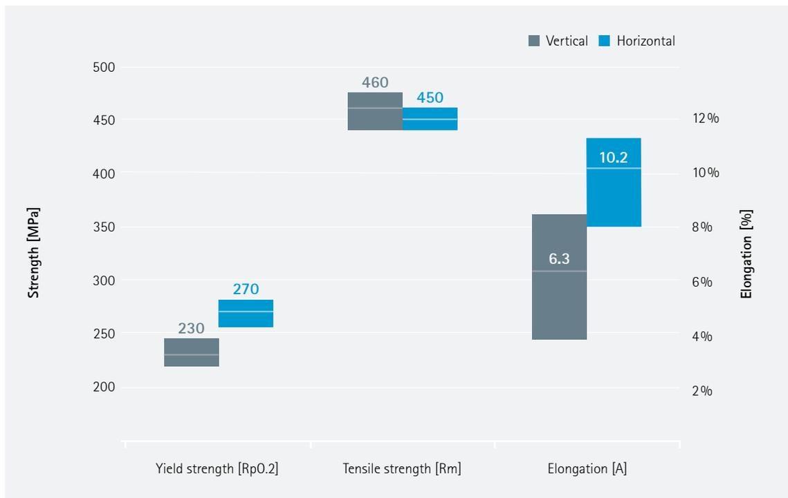
The testing was done according to ISO 6892-1, B10. Machined (turned) samples were used.
