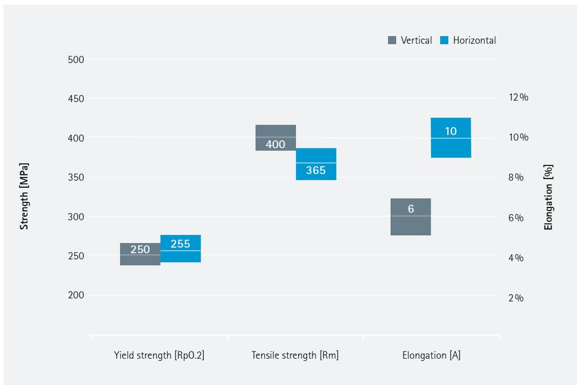
The testing was done according to EN 2002-001 2005 on round specimen machined according to standard Annex C. Results of both horizontal and vertical building direction are presented.
