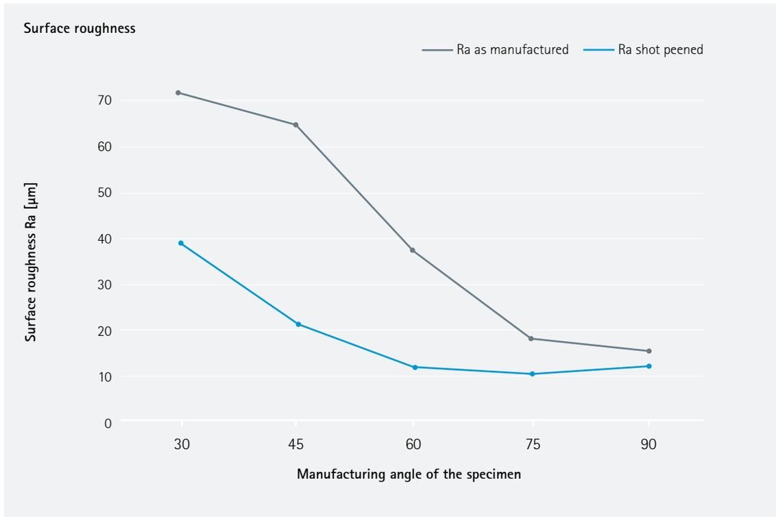
The surface quality was characterized by optical profiling from down-facing surfaces according to internal procedure. The 90 degree angle corresponds to vertical surface.
