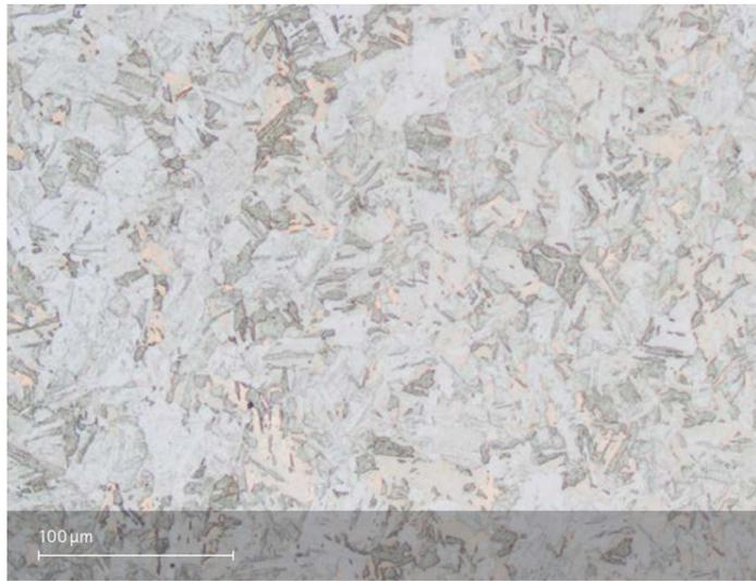
Heat treated microstructure. Etching; ASTM E407-94
