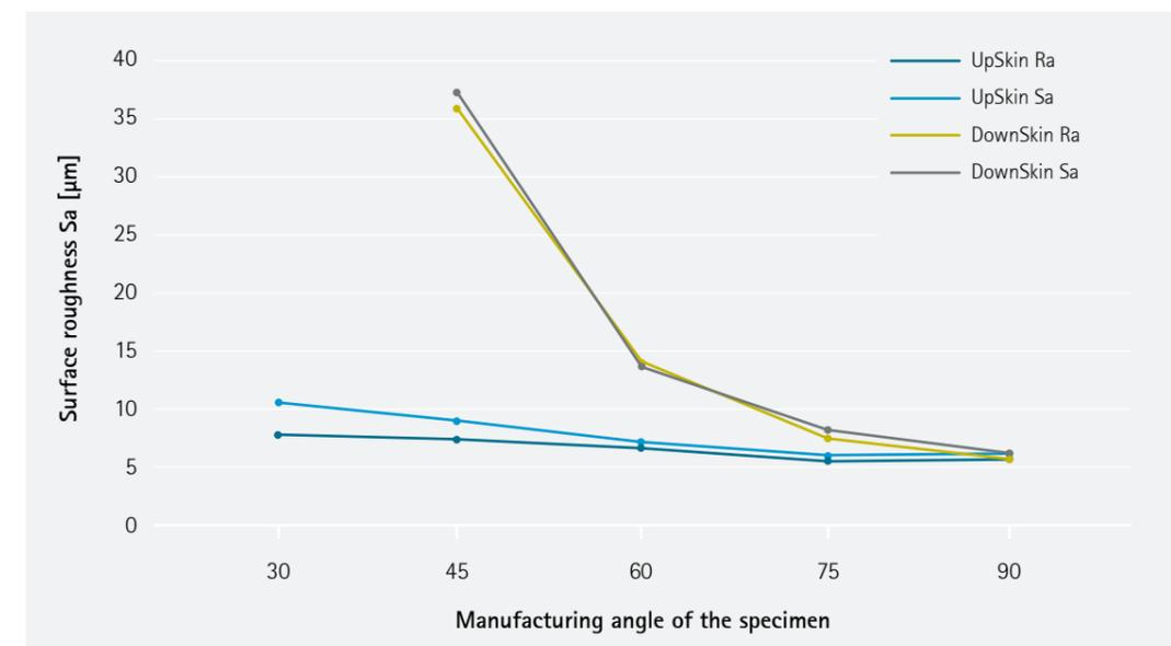
The surface quality was characterized by optical measurement method according to internal procedure. The 90 degree angle corresponds to vertical surface.
