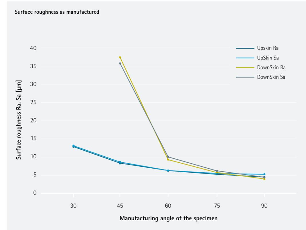
The surface quality was characterized by optical measurement method according to internal procedure. The 90 degree angle corresponds to vertical surface.
